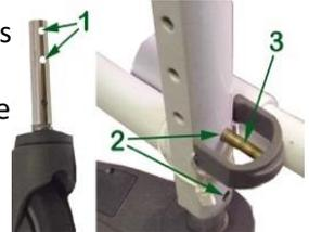
4. Insert the anti-tippers into the two anti-tipper receiver tubes located at the rear of the frame above the casters.
