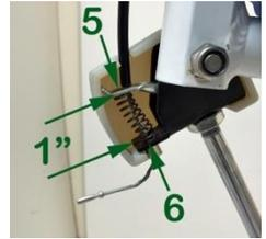
If the chair angle cannot be changed when the tilt lever (4) is pressed the cause is usually out of adjustment or stretched cables. If the chair will not lock at any angle the cables are likely adjusted too tight.
