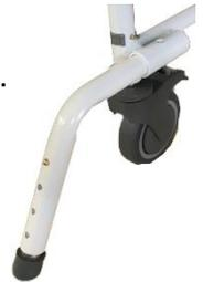
5. The adjustment is made by simply depressing the anti-tipper push pin (1), sliding the inner anti-tipper tube (2) to the desired length, aligning the push pin with the closest adjustment hole (3) and allowing it to pop through.
