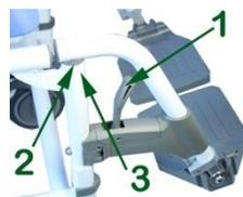
To replace the footrests, lower the footrest pivot plug (2) into the commode seat frame holes (3) from the side on the center of the seat and swing the footrests to the front until they lock into position.
