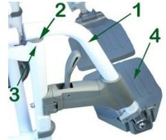
7. The foot plate height can be adjusted by loosening the footrest clamp (1), sliding the foot plate extension tube (2) up or down inside the footrest hanger tube (3) and re-tightening the clamp.
