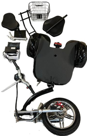
2.) Place your Chaser 1000 on a flat, clean surface. Place a block 3.5” under the front, by the battery. This will make it easier for the next step.
