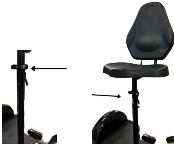
**WARNING:** Do not attempt to adjust the seat during operation. Always remove the key before adjusting. Failure to do so could result in personal injury or damage to the equipment.
