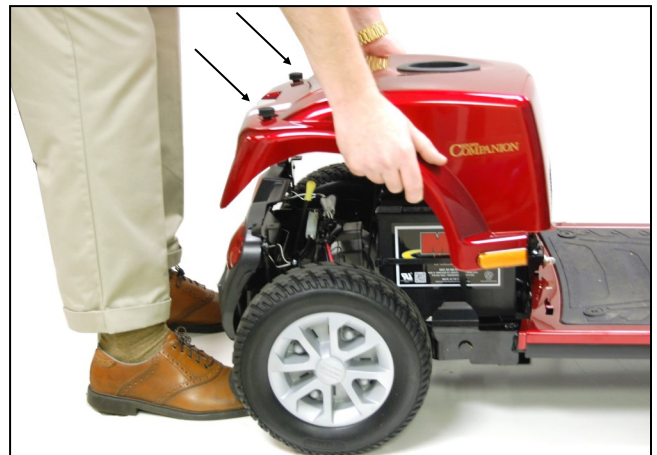
FIGURE 16. REMOVING THE REAR SHROUD
