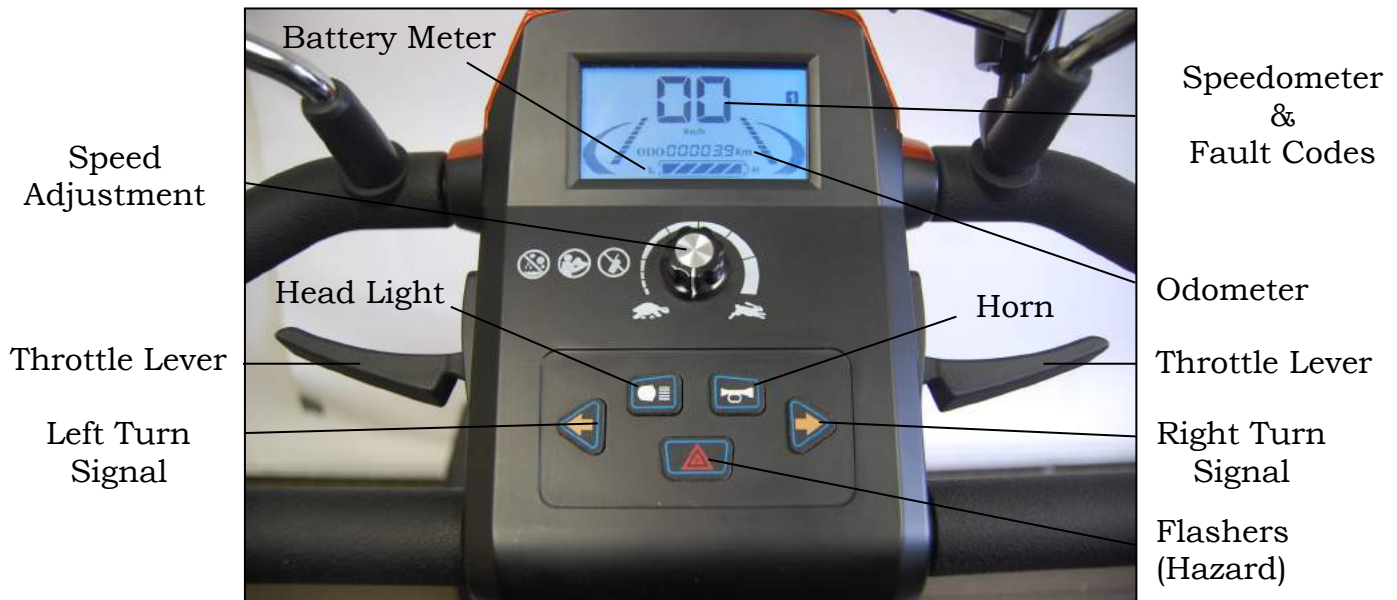
Figure 5. Delta Tiller Control Panel with LCD Display
