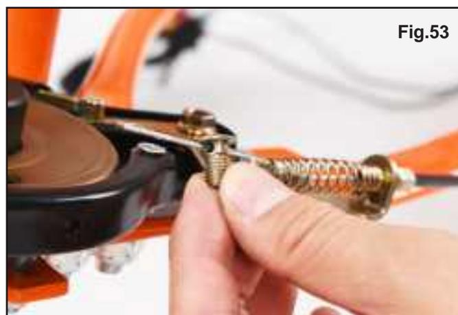
8) Press and hold the rear brake lever forward, at the same time, tighten the nut firmly (Fig.54). Example of rear brake assembly is as (Fig.55). After adjust the brake, clip the wire cap at the brake cable end.
