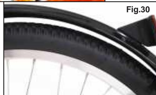
3) Rotate the rear wheel until there is adequate space for the Phillips Head screwdriver to reach through the spokes to the fender hole. Fasten a screw through the center fender hole into the center hole of the rear frame (**Fig.31**).
