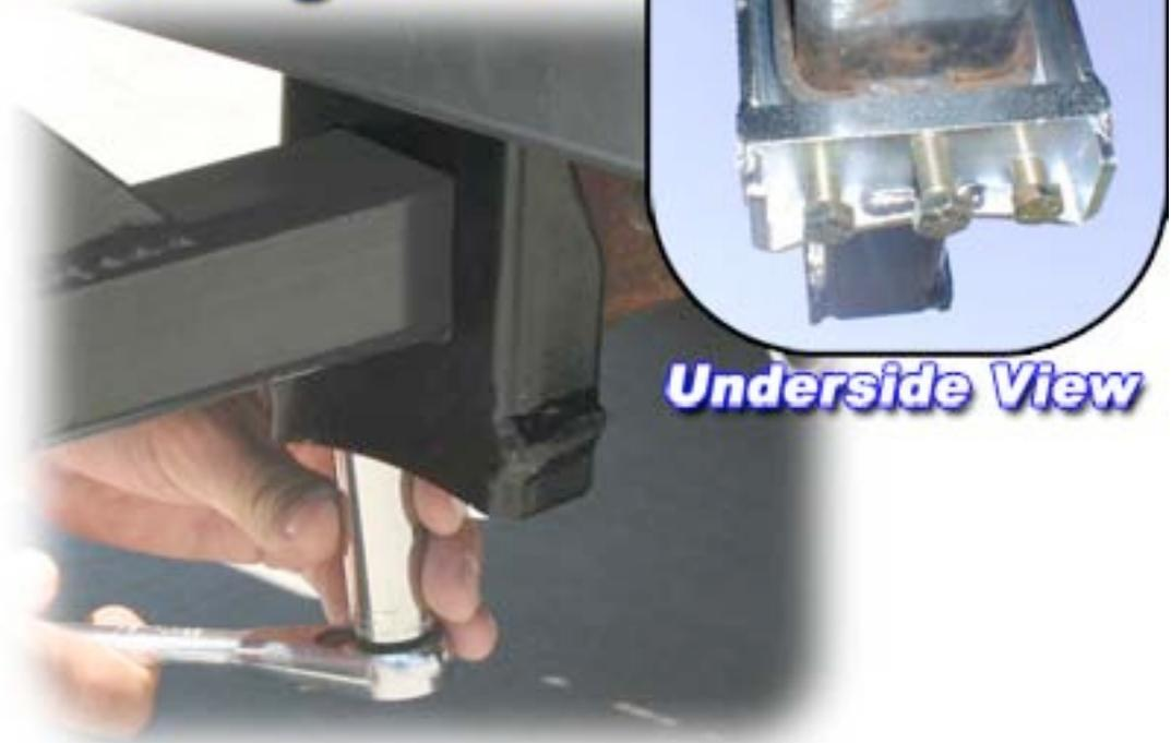
Next loosen the bolts on the anti-tilt lock bracket. (There should be grooves where the bolts were tightened against the hitch receiver)
