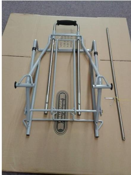
**Insert the wheel axle through the body of the frame. You will notice the axle has three holes. With your frame positioned as pictured above, slide the side of the axle that has the two holes into the frame. The side with the two holes must be on the right side of your cart.**
