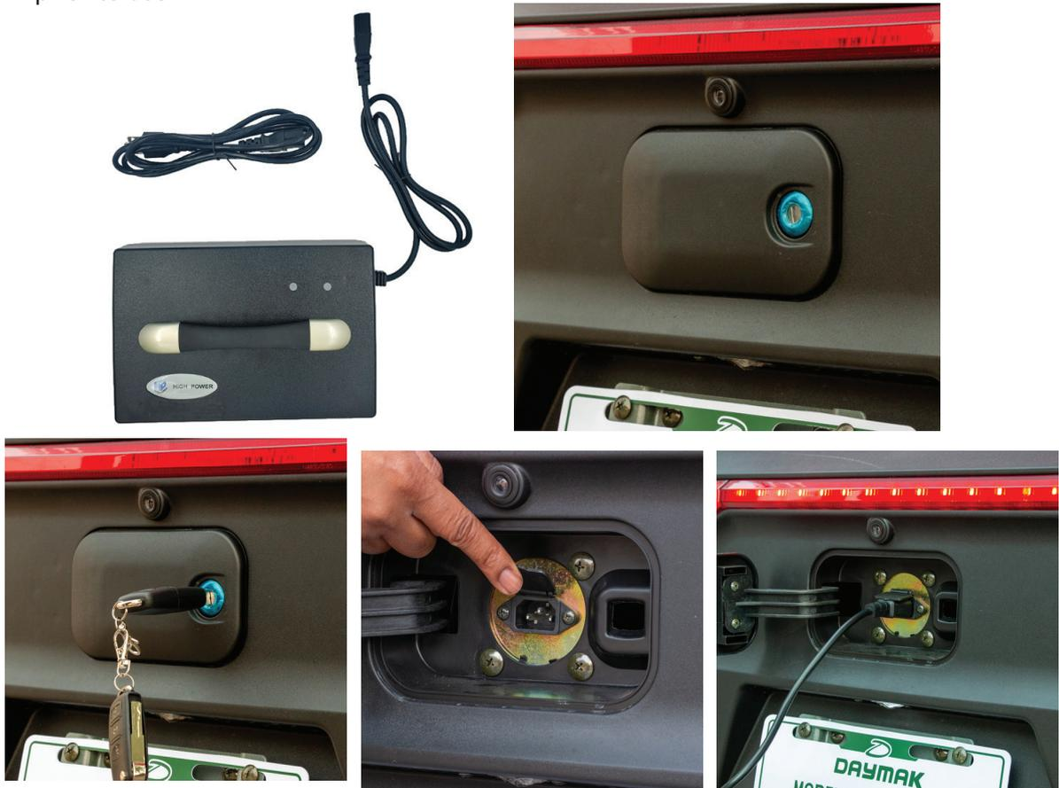
To access the charge port, take the keys and at the back of the unit unlock the charge port door. Inside you will find a plug. Lift up the cover and plug the charger into the socket.
