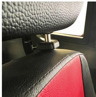
Look for the button under the left mounting rod (left as if you are sitting on it) and while holding that button in with your hand, raise or lower the head rest to your desired height.
