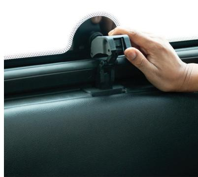
Then push the window open with your hand and while pushing the window open clamp the latch down to hold it in place.
