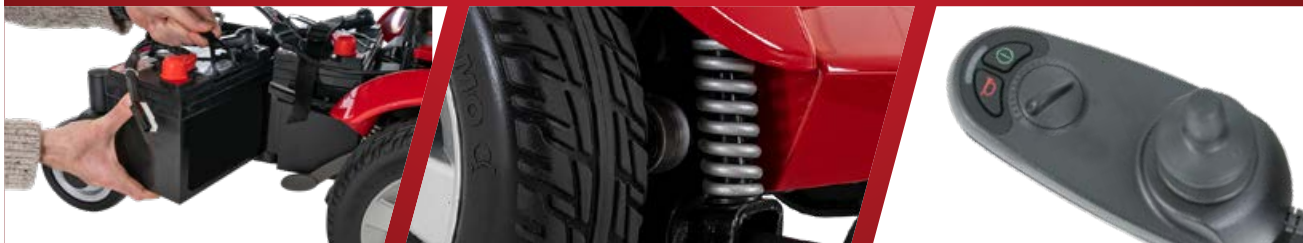
Side access to the battery
