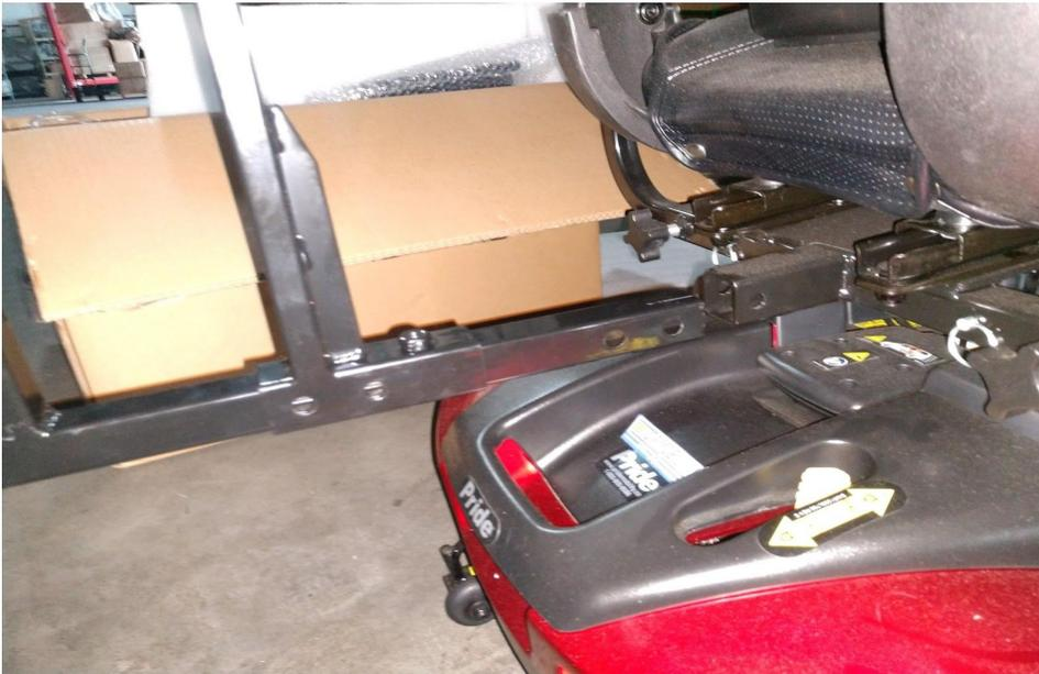
Use the Velcro in the center of the Vertical bar to keep the Walker from bouncing.
