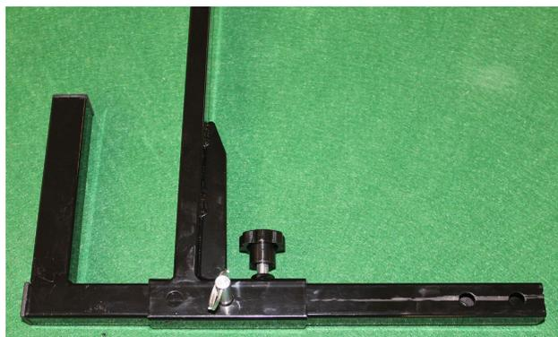
Insert the Upper Bar into the Vertical bar. Secure this in place with a Tension Knob (either way).
