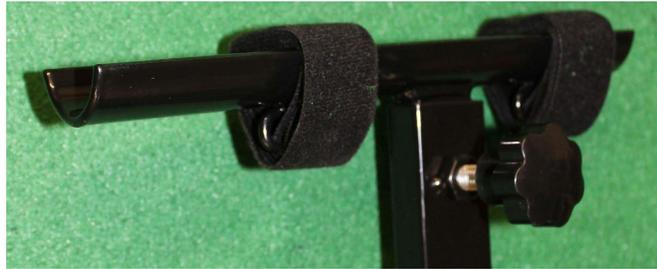
Adjust the Vertical Bar to the center of the Mount Bar. Pin this in place with a Clevis Pin. Secure this in place with a Tension Knob.
