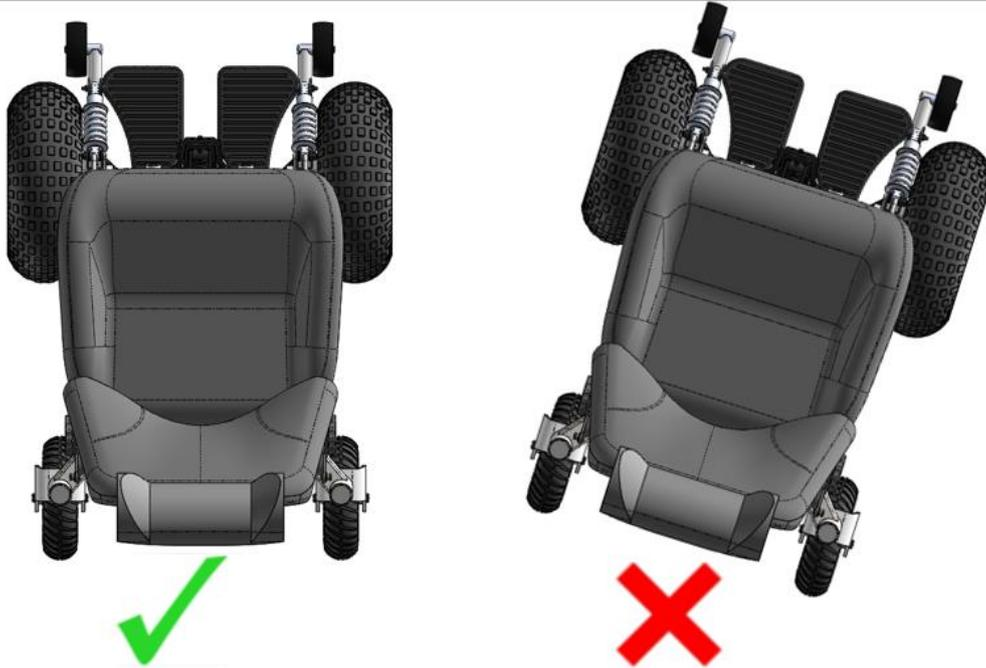
Figure 6 - Frontier V4 FWD Correct and Incorrect Approaches to Obstacles
