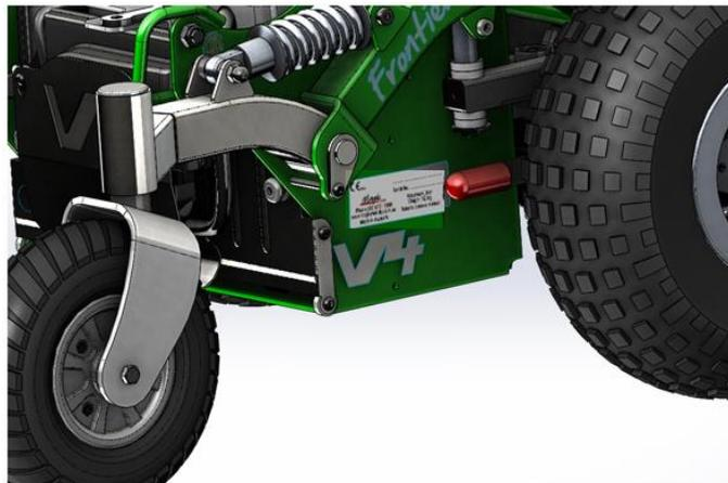
Figure 3 - Frontier V4 Serial Number Location
