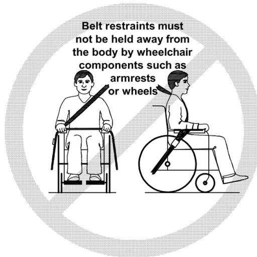
Figure 13 - Improper belt restraint fit
